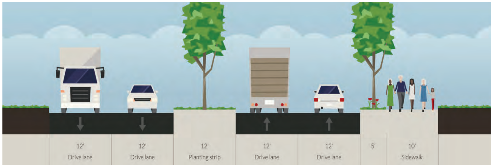
Figure: Section view of the corridor looking west, as proposed.
