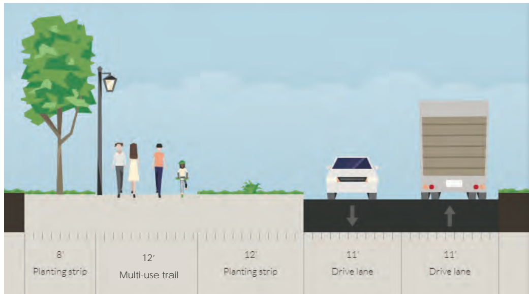
Figure: Section view, looking north, with trail on west side of ROW.
