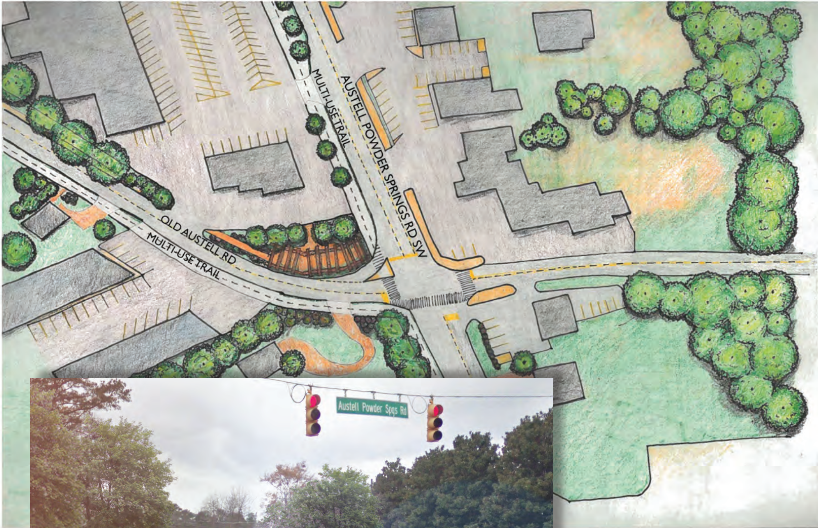
Left: Rendering of proposed improvements, looking west towards Old Austell Road from Austell-Powder Springs Road. Elements include a raised pedestrian island, new crosswalks, sculptural placemaking elements and multi-use trail on Old Austell Road.
